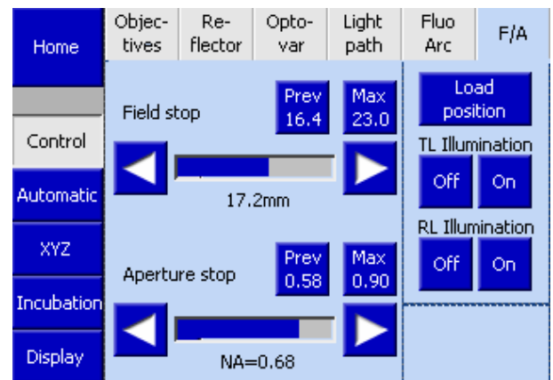
Fig. 4-35 Page Microscope -> Control -> F/A
